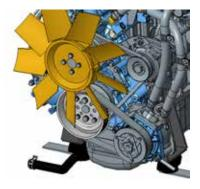
When sudden transient response is required from external loads (i.e. pumps, motors or other electrical devices) the generator controller quickly deactivates the electric clutch in order to allow generator to provide 100% of generator output power to connected electrical devices.
