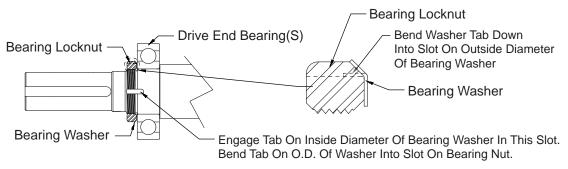
Some pumps are equipped with double angular contact bearings at the drive end. It is imperative that these bearings be installed in the correct orientation relative to one another. When installing the first of the two angular contact bearings onto the shaft make certain that the side of the inner race with the largest diameter is located against the shaft shoulder. The next bearing must be installed with the smaller diameter side of the inner race against the first bearing.
