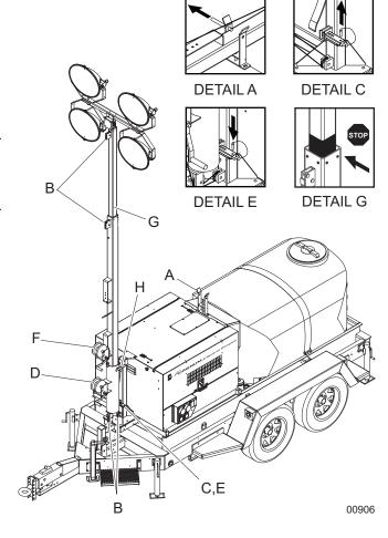
6. After the mast is up and locked into place, use the upper mast winch (F) to telescope the mast to the desired height. Extend the mast slowly, making sure the electrical cord is extending at the top sections of the mast. If, for any reason, the winch cable begins to develop slack or any of the mast sections get stuck, **STOP**IMMEDIATELY and contact an authorized service center.
