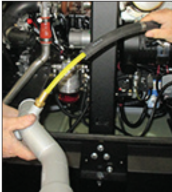
Figure 12 - Heat Cable Through PCV Hose—No Yellow Visible
