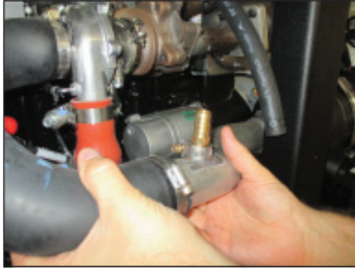
Figure 4 - Detaching Hoses, Removing Weldment
