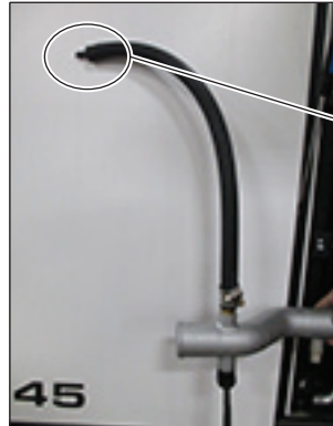
Figure 12 - Heat Cable Through PCV Hose—No Yellow Visible
