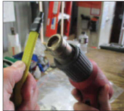
Figure 11 - Shrink End-Cap to Cable
