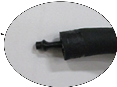
Figure 12 - Heat Cable Through PCV Hose—No Yellow Visible
