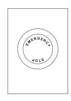
The switch will remain closed until it is pulled out.
