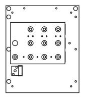
LINK BOARD ATTACHED IN 208 VOLT 3Ø POSITION
