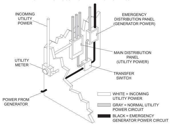
Installation of a transfer switch or other type of remote starting device is the responsibility of the generator user. Installation of such devices must be performed by following all directions supplied by the manufacturer of the switch. If attaching the generator to a power supply normally serviced by a utility company, notify the utility company and check local and state regulations. Familiarize yourself with all instructions and warning labels supplied with the switch.
