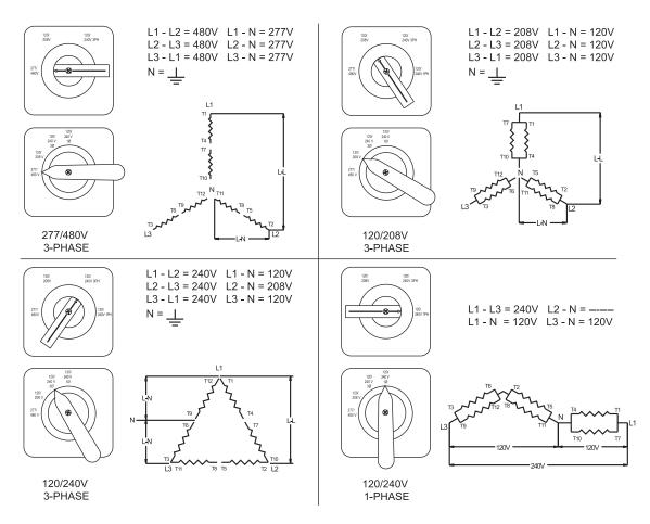
The voltage selector switch is equipped with a locking mechanism. Once the proper voltage has been selected, push the red latch on the inside of the switch handle up and insert a padlock through the handle. By locking the handle in place you will prevent unauthorized personnel from changing the switch settings.
