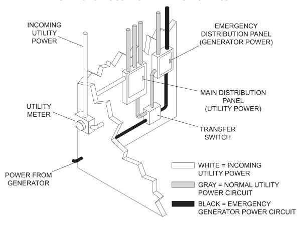
Installation of a transfer switch or other type of remote starting device is the responsibility of the generator user. Installation of such devices must be performed by following all directions supplied by the manufacturer of the switch. If attaching generator to a power supply normally serviced by a utility company, notify the utility company and check local and state regulations. Familiarize yourself with all instructions and warning labels supplied with the switch.
