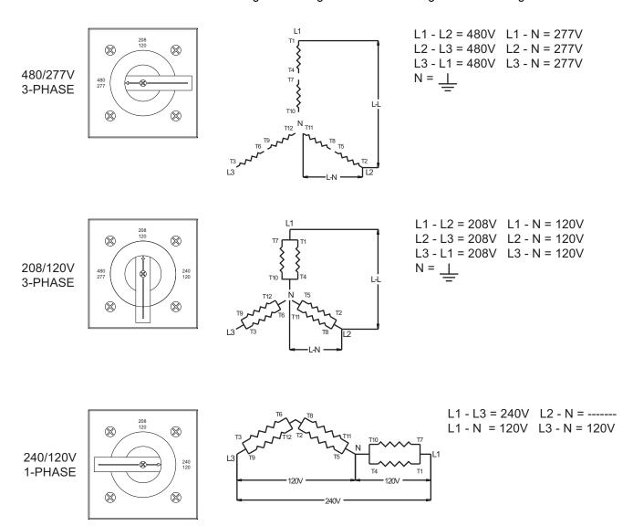
The voltage selector switch is equipped with a locking mechanism. Once the proper voltage has been selected, push the red latch on the inside of the phase switch handle up and insert a padlock through the handle. By locking the handle in place, you will prevent unauthorized personnel from changing the switch settings.
