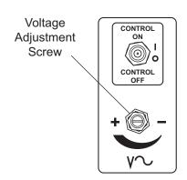
The output voltage of the generator may be adjusted after the generator is running by using the fine voltage adjustment screw. The adjusting screw is located directly below the "CONTROL ON/OFF" toggle switch on the control panel.
