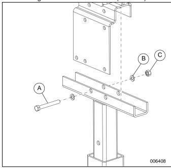
Figure 12. Bracket/Light Fixture Installation to Mast
