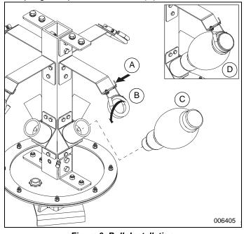
Figure 9. Bulb Installation
