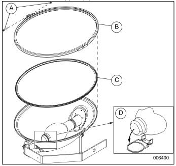
Figure 4. Bulb Removal
