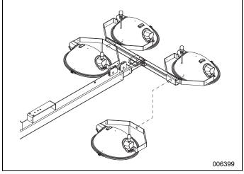
Figure 3. Light Fixture Removal
