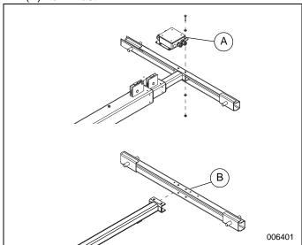
Figure 5. Junction Box and Crossbar Removal
