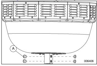
See Figure 10. Install bearings (A) to light fixture.
