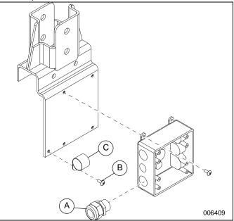
Figure 13. Junction Box Installation
