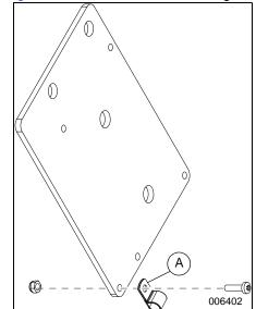
Figure 6. Tubing Clamp Removal
