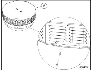
Figure 7. Hardware Removal—Side of Lid
