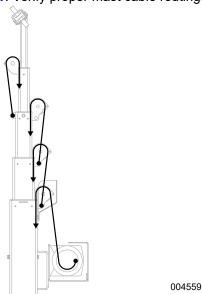
Figure 4-1. Proper Mast Cable Routing
