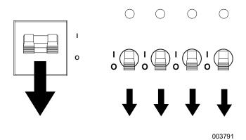
Figure 3-4. Circuit Breakers in OFF (O) Position
