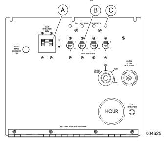
Figure 3-8. Light Switches and Breaker
