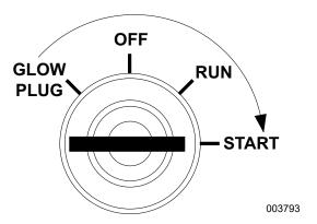
Figure 3-6. Crank Engine
