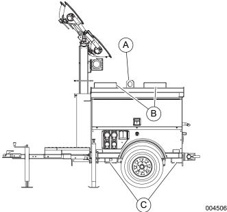
Figure 3-13. Lifting Point
