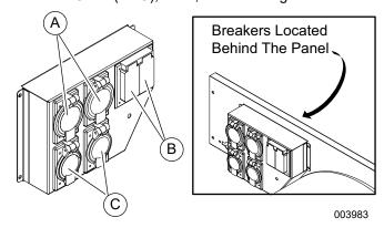
Figure 3-9. Auxiliary Outlets
