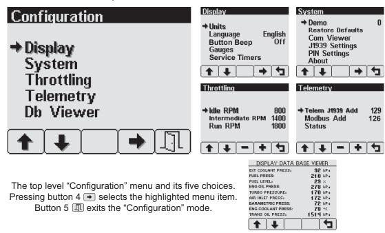
**Note:** Most configuration changes take effect immediately. Some such as Idle RPM take effect on the next power up.
