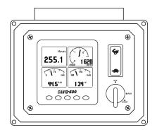
If the ECU is preheating when the key switch is turned to the "RUN" position, a Preheat screen will appear. Preheat time varies with atmospheric and engine conditions. After waiting for the Preheat screen to extinguish, the engine is cranked by turning and holding the key switch in the "START" position until the engine starts.
