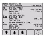
Example alarm message, alarm list screens showing unacknowledged conditions and acknowledged alarms. After acknowledgement, the Exit button  $|\mathbb{I}|$  becomes active.
