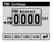
If the two PINs do not match, an error message is displayed and the PIN is unchanged.
