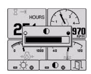
**Note:** The display adjusts the contrast with ambient temperature. Manual contrast adjustments are only necessary with extreme climate change.
