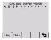
Button 1 sop freezes the display while button 2 solves shows CANbus data statistics screen.
