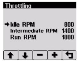
The "Throttling" menu allows programming the automatic start/stop throttle profiles.
