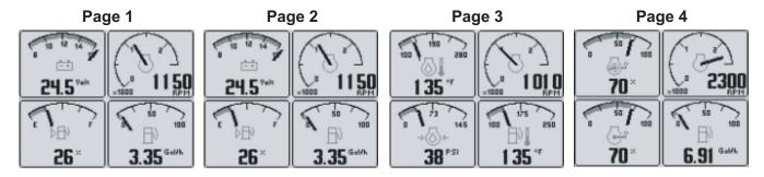
**Note:** Engine hours are displayed as a digital value even on Analog Gauge Pages. The default gauge pages represent 13 selections since the tachometer is repeated in the upper right quadrant of each page.
