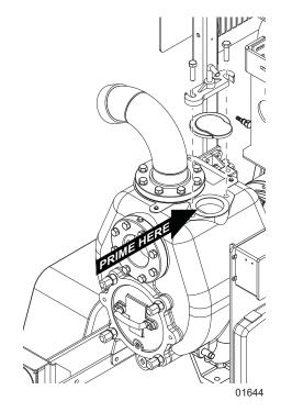
Figure 12 - Remove Priming Cover
