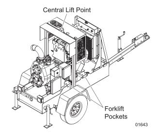
Figure 18 - Lifting Points
