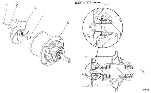
Figure 26 - Impeller Components
