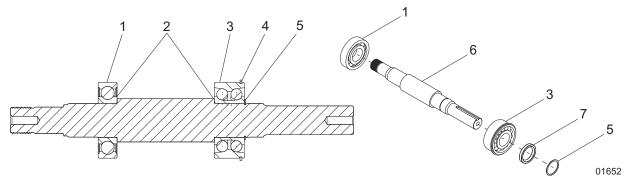
Figure 22 - Bearing/Shaft Assembly
