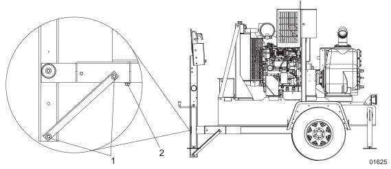
Figure 5 - Removing the Shipping Brace
