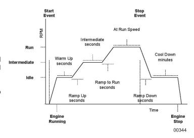
Figure 9 - Throttle Control Profile
