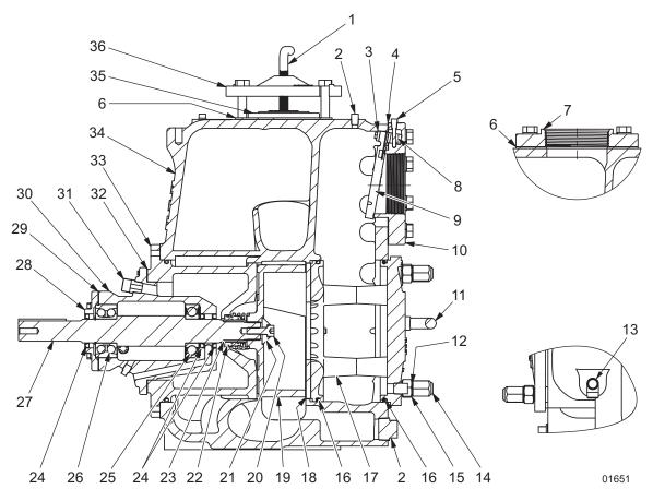
Figure 21 - Self-Prime Pump Cross-section
