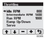
**Note:** The minimum engine speed is set by the ECU. Requesting a lower speed causes the engine to run at the ECU minimum speed. RPM limits are programmed into the panel to limit the requested speed. Contact Generac Mobile Products for information on changing the panel minimum requested RPM and maximum requested RPM.
