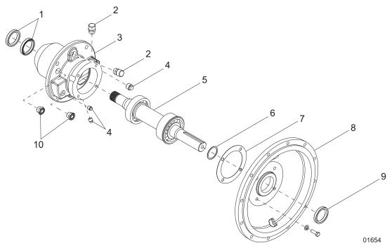
Figure 23 - Bearing Frame Assembly
