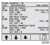
The examples above are alarm list screens showing unacknowledged conditions and acknowledged alarms. After acknowledgment, the exit button becomes active.
