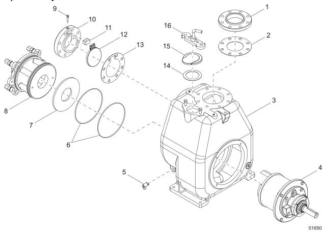
Figure 20 - Self-Prime Pump Assembly
