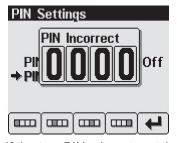
If the two PINs do not match, an error message is displayed and the PIN is unchanged.
