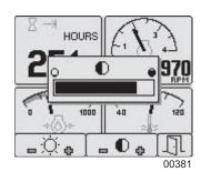
The menu is exited by pressing button 5 . The lighting and contrast settings are retained after the unit is powered off.
