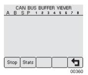
Button 1 stop freezes the display while button 2 states shows the CANbus data statistics screen.
