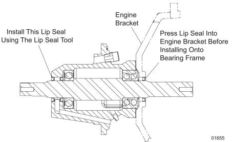
Figure 24 - Installing the Lip Seals
