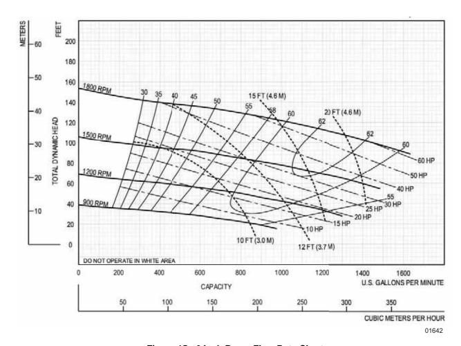
Figure 15 - 6 Inch Pump Flow Rate Chart
