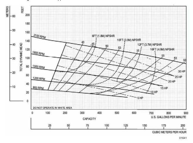
Figure 14 - 4 Inch Pump Flow Rate Chart
