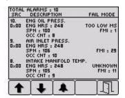
In the examples above are alarm list screens showing unacknowledged conditions and acknowledged alarms. After acknowledgement, the exit button  $|\Pi|$  becomes active.
