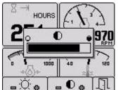
The menu is exited by pressing button 5 . The lighting and contrast settings are retained after the unit is powered off.
