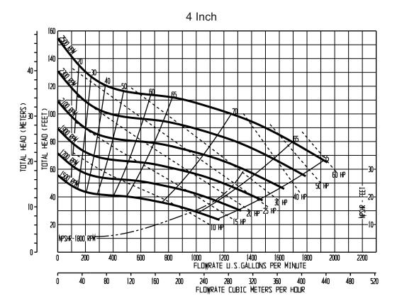
Note: Performance includes losses for check valve, priming system and open clearance wear ring.
