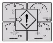
Pop-up warnings of service required and data communications failure.
