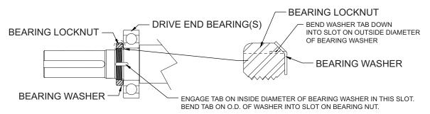
Some pumps are equipped with double angular contact bearings at the drive end. It is imperative these bearings be installed in the correct orientation relative to one another. When installing the first of the two angular contact bearings onto the shaft, make certain the side of the inner race with the largest diameter is located against the shaft shoulder. The next bearing must be installed with the smaller diameter side of the inner race against the first bearing.
