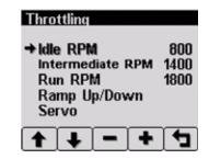
**Note:** The minimum engine speed is set by the ECU. Requesting a lower speed causes the engine to run at the ECU minimum speed. RPM limits are programmed into the panel to limit the requested speed. Changing the panel Minimum Requested RPM and Maximum Requested RPM requires using the CANplus Configurator.
