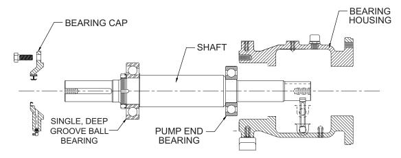
On the drive end of the bearing housing, remove the capscrews holding the bearing housing cover or the SAE bracket to the housing. Gently slide the housing cover or the SAE bracket off of the shaft to protect the lip seal(s) if it is to be reused.
