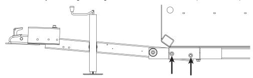
**Note:** If the jack was used to support the unit while removing the shipping brace, the jack must be moved back to the tongue location before the unit can be towed. Connect the trailer tongue to a vehicle or other support and move the jack to the tongue location.
