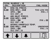
Example alarm message, alarm list screens showing unacknowledged conditions and acknowledged alarms. After acknowledgement, the exit button  $[\Pi]$  becomes active.
