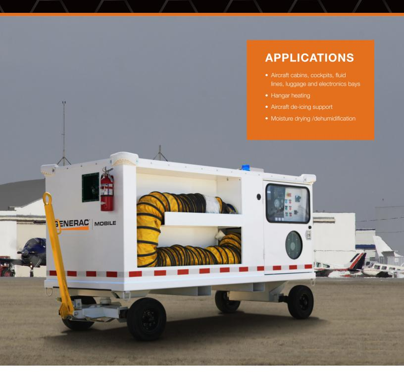
Compact and portable, Generac Mobile heat carts provide clean and reliable heat for aircraft, hangars and ground support equipment (GSE). Our heat carts are designed with the latest in burner, fuel flow and airflow technology. Heat carts deliver reliable heat and performance in extreme low temperatures down to -50°F/-45°C.
